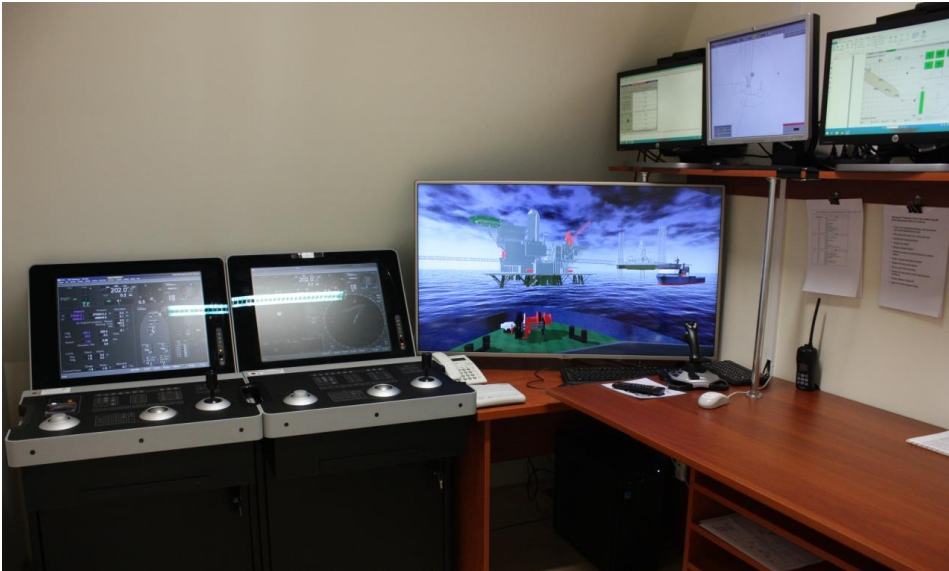
Fig. 6. DP simulation system with thrusters' allocation and vision prepared in MUS
