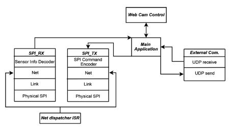
Figure 5. PC104 Software Architecture
