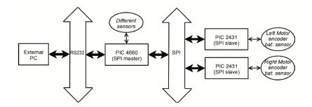
Figure 2. ExaBot architecture without the PC104
