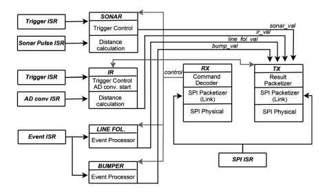
Figure 3. PIC18F4680 Software Architecture
