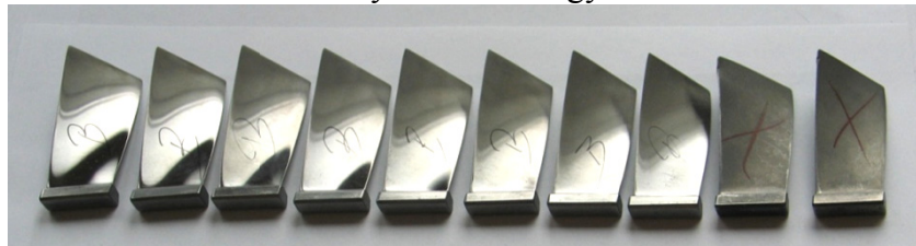
Fig. 1. Blades of the 1-st stage compressor retired from maintenance under technical inspection of engine, destined for fatigue test.
