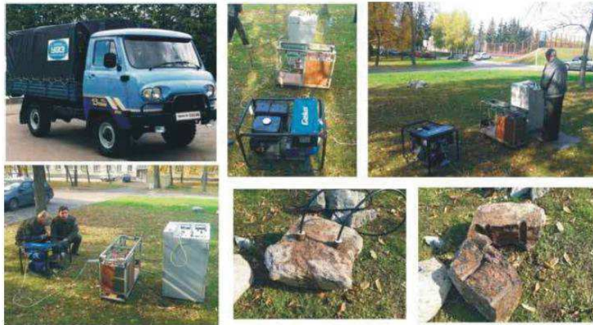
Fig. 13. Loosening the rock blocks by the EHD method [24]
