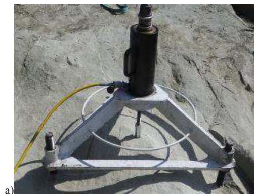
Fig. 17. Own tests on mechanical loosening of rocks within the RODEST project: a) test stand equipment, b) determination of maximum force ( F_{max} ), recorded during the loosening test [33]
