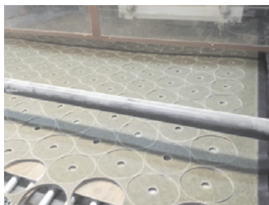
Fig. 2. View of the location designed for cutting disks out from glass meshes saturated with PF composition
