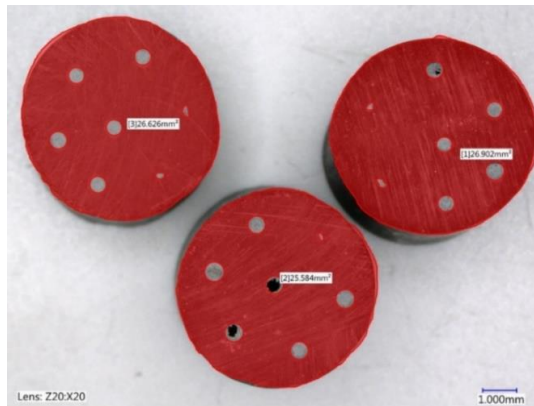
Fig. 4. Measurement of the cross-sectional area of specimens [12]
