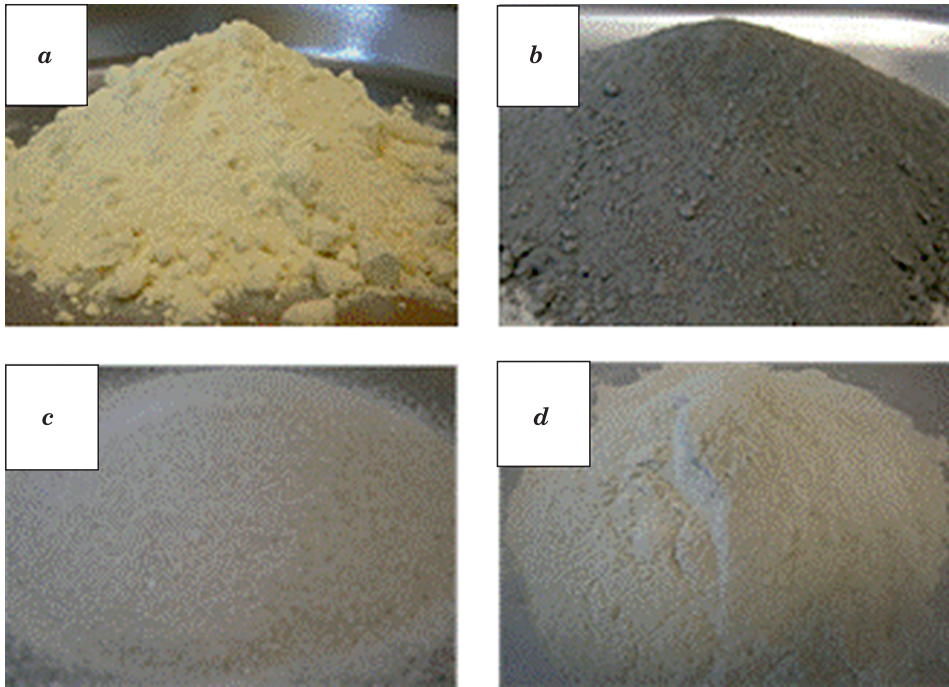
Fig. 1. Materials used in the researches: a - sulphur, b - fly ash, c - microsilica, d - zeolite Source: Fig. b - Photographs taken by D. JANKOWSKI
