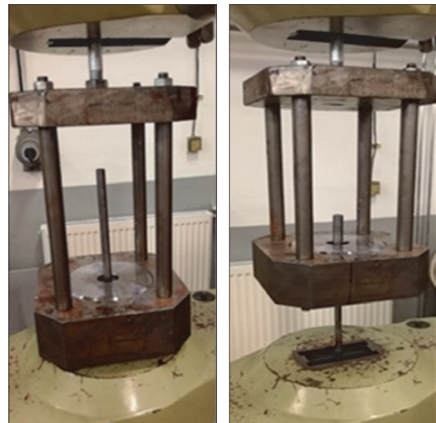
Fig. 2. Detail of the special fixture clamped in the universal hydraulic tensile testing machine EU 40
