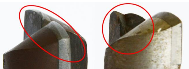
Fig. 2. Examples of drill bit wear
