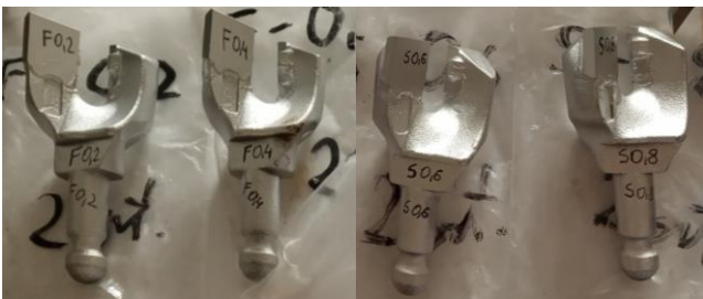
Fig. 6. Photos of sample drill bits F and S before testing
