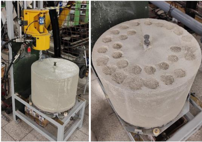
Fig. 5. Station with a sample before and after testing
