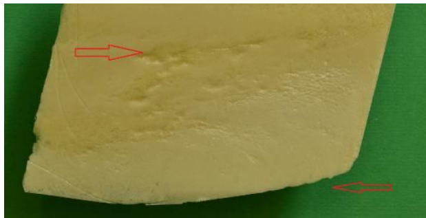
Fig. 5. Test casting of a wing length with evident defects on the surface and at the trailing edge
