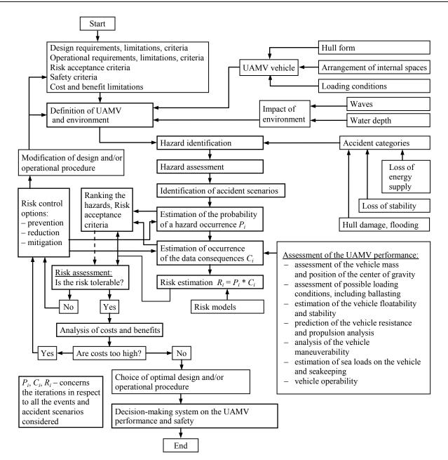
Figure 2. Structure of the method for assessment of the UAMV performance and risk assessment
