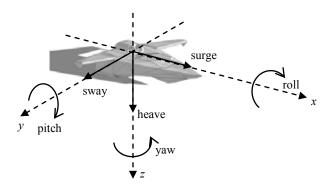
Figure. 5. Standard model using 6 DOF
