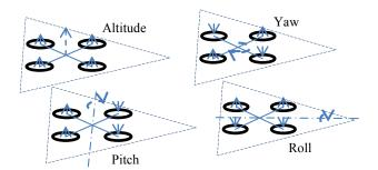
Figure. 4. Thrust vectors of the precise propulsion units during the UAMV vehicle positioning
