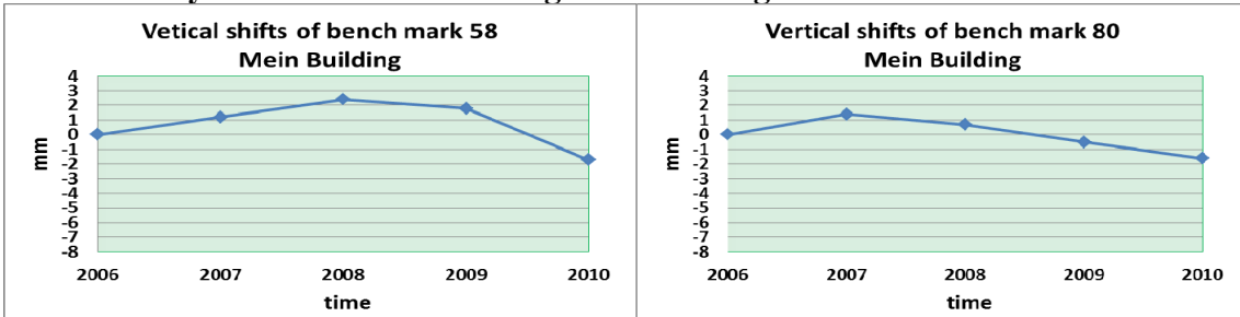
Rys. 5. Vertical shifts of bench mark of Mein Building.
