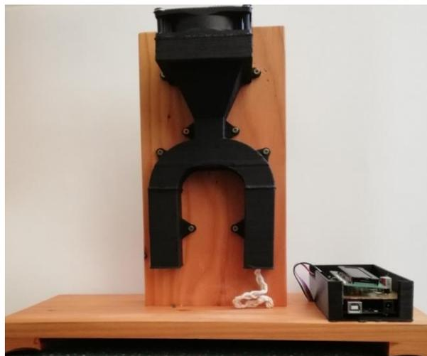
Fig. 6. Aspiration psychrometer based on digital temperature measurement
