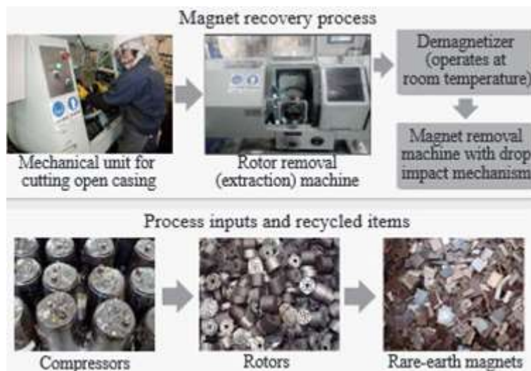
Fig. 3. Process Used to Separate and Recover Rare-earth Magnets from Air Conditioners (Source: Baba et al. [5])
