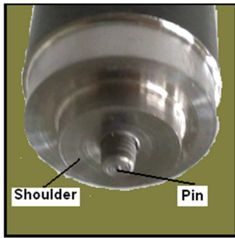
Fig. 2. Mixer pin used in FSW
