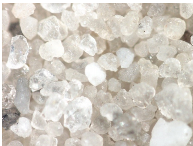
Fig. 4. Micrograph of foundry 4 sand reclaimed in 550 °C
