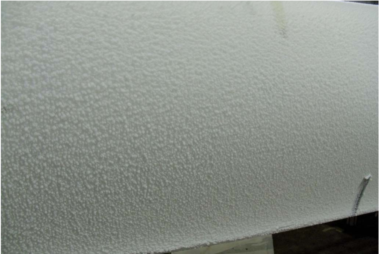
Fig. 9. Snowflakes ice type formed during the tests
