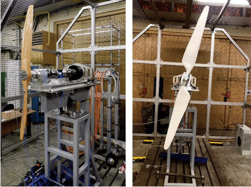
Figure 10. Tests' propellers: commercial wooden Aerobat (left), and carbon composite from the Łukasiewicz – Institute of Aviation (right).
