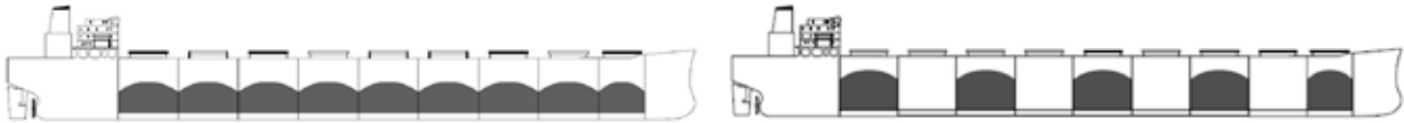
Figure 1. A homogeneous hold loading condition and an alternate hold loading condition (IACS, 2018)
