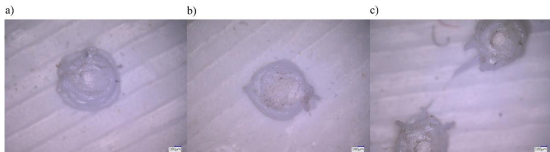
Figure 5. The microscopic images of Braille dots taken and magnification 100× (a) dot in letter “j”, (b) dot in letter “z” (c) stringing between dots
