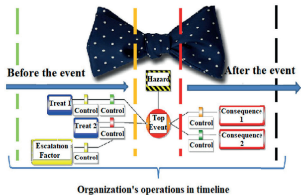
Fig. 2. Diagram showing the operation of the BowTie method [27]
