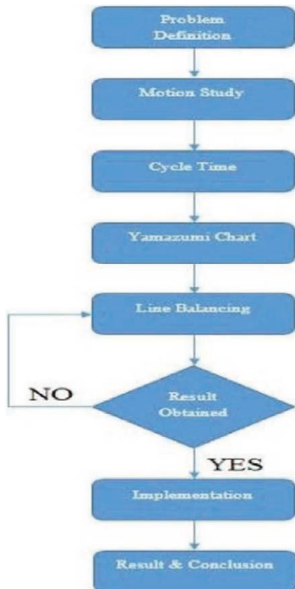
Fig. 2. Line balancing methodology [12]
