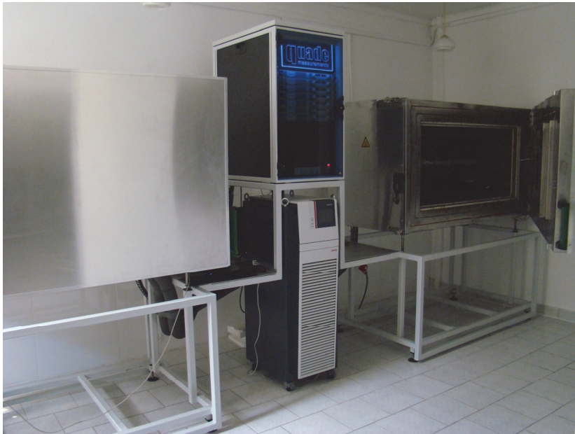
Fig. 3. The two-chamber pipe apparatus for thermal conductivity tests within the temperature range from -40 to 600^{\circ}\text{C}
