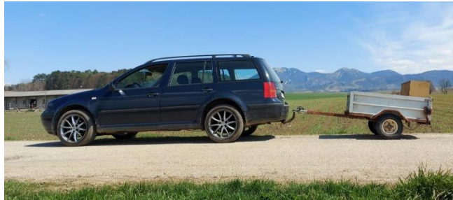
Fig. 10. A real vehicle-trailer combination with the load deposited in the rear part of the trailer
