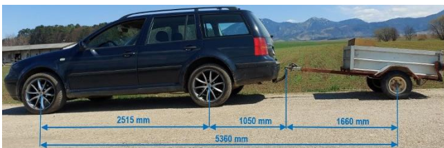
Fig. 2. Dimensions of the vehicle–trailer combination
