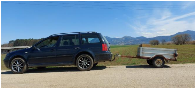
Fig. 6. A real vehicle–trailer combination with the load deposited in the front part of the trailer
