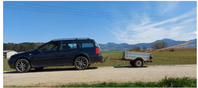
Fig. 13. A real vehicle-trailer combination with the CoG of the load situated behind the trailer
