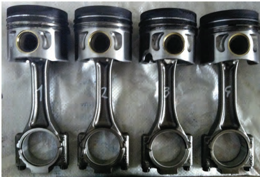
Fig.7. The view of the piston groups after the tests
