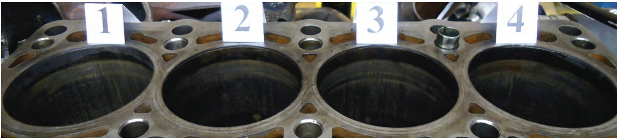
Fig.6. View of the engine block after test, removing the pistons and removing deposits
