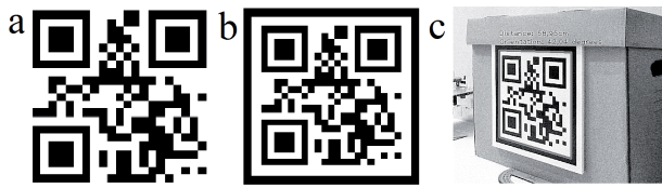
Fig. 5. Exemplary QR code based landmark: QR code encoding value '1' (a), 16.5x16.5 cm landmark with frame (b), recognized landmark in the environment (c)
