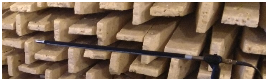
Figure 7. Measurement nosecone with the suitable probe-tube shielding mounted on the measurement microphone.
