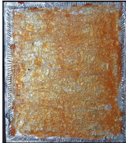
Fig. 5. Wax added to the wooden mold ( own photo )
