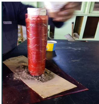
Fig. 3. Resin added in external mold ( own photo )
