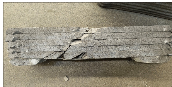
Figure 8. Automatically reinforced beam (sample no. 41RT) after three-point bending test
