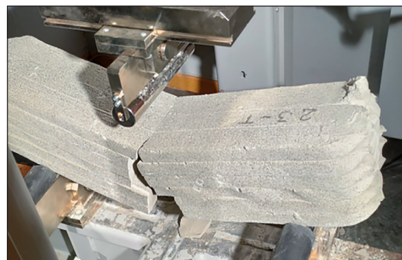
Figure 5. The beam without reinforcement (sample no. 23-T) destroyed in the bending process
