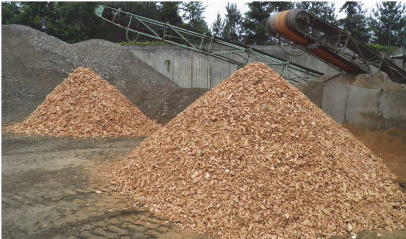
Fig. 1.4. Ready to use waste ceramic aggregate (photo by J. Katzer)
