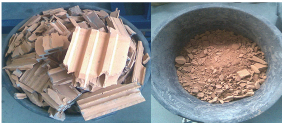
Fig. 2.1. Ceramic waste and ground ceramic waste [12]
