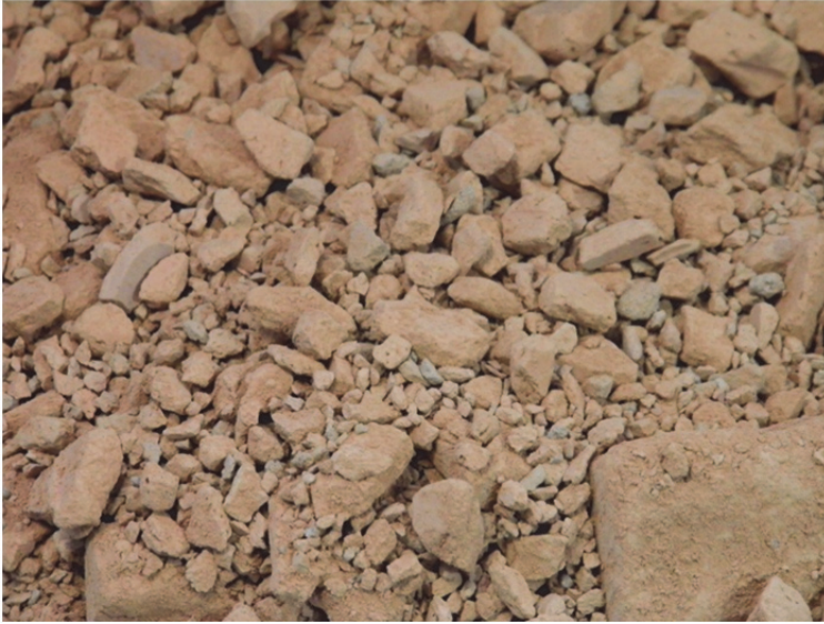
Fig. 2.3. Ground ceramic waste used as coarse aggregate[11]
