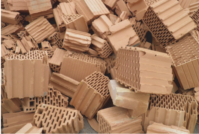
Fig. 1.3. Ceramic waste from construction industry (photo by J. Katzer)
