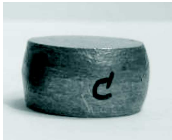
Fig. 4. lead cylinder after deformation by "Barrel Compression Test" for measurement of the friction coefficient
