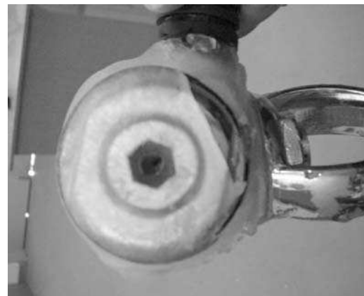
Fig. 4. Icing of the 1 st stage of a regulator.
