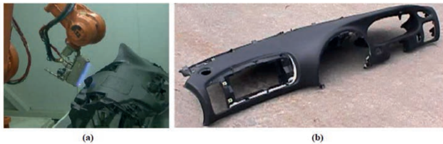
Fig. 8. SICOR treatment of automotive TPO instrument panel (IP): (a) flame treatment prior to spray-application of PEI-based primer, and (b) IP after vacuum wrapping
