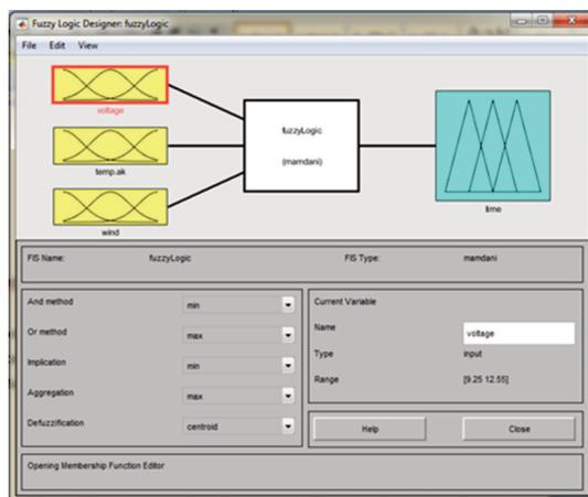
Fig. 6. Decision making system in MatLab Fuzzy Logic.
