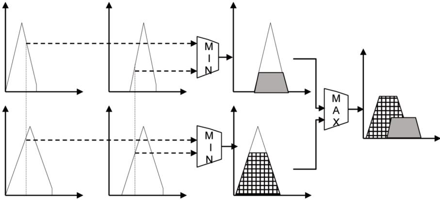
Fig. 5. Strategy for calculating an array of fuzzy conclusions by the Mamdam method.
