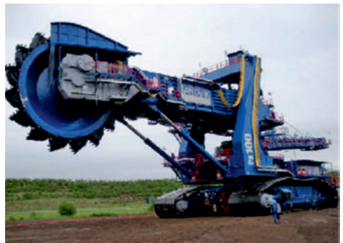
Rys. 8. Koparka kompaktowa SANDVIK PE100 [20] Fig. 8. Compact BWE Type PE 100 (built by Sandvik)
