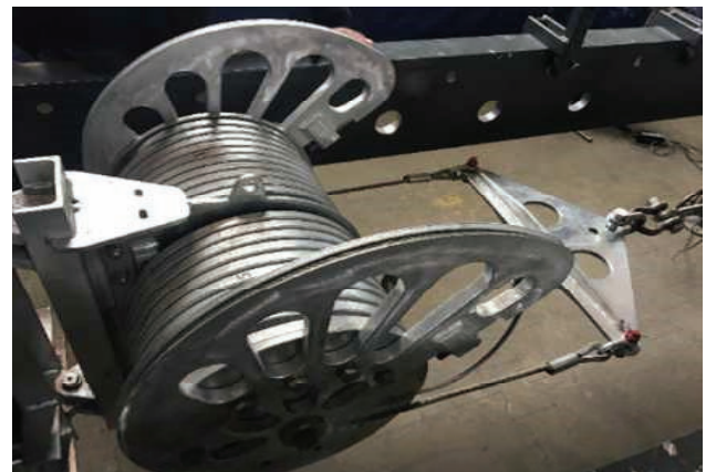
Fig. 2. Spring tensioning device [photo: P. Kwaśniewski]
