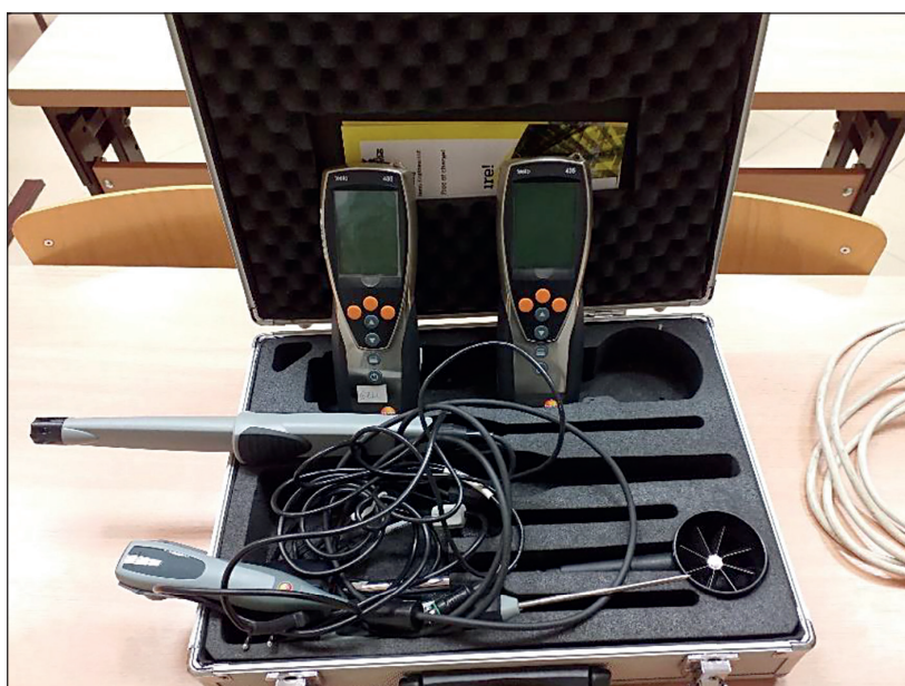
Fig. 4. Measuring instrument with probe air quality and probe carbon monoxide
