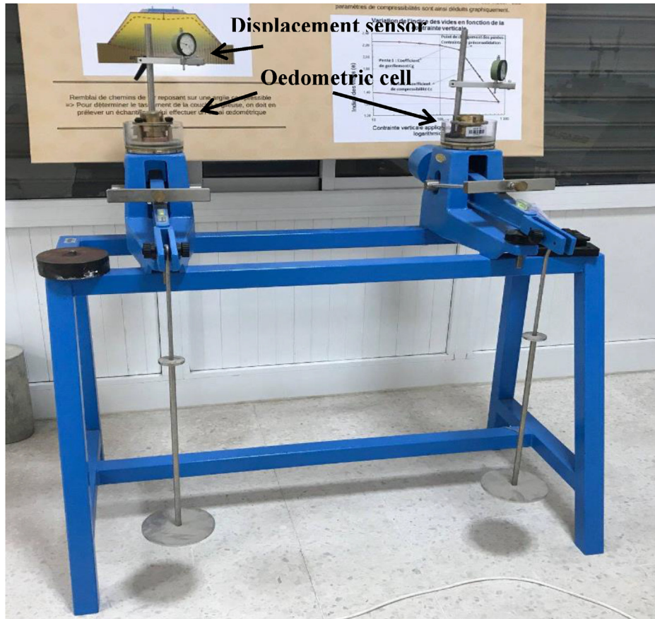
Fig. 7. Photo corresponding to the first step of the sample's disposition before oedometric compressive loading.
