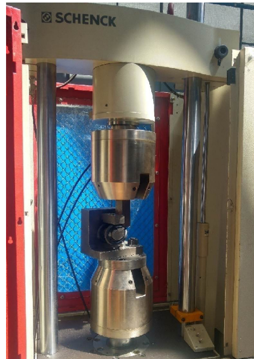
Fig. 3. Sinus 250 strength testing machine with SB4-type spring clip clamping force testing equipment [authors' own work]
