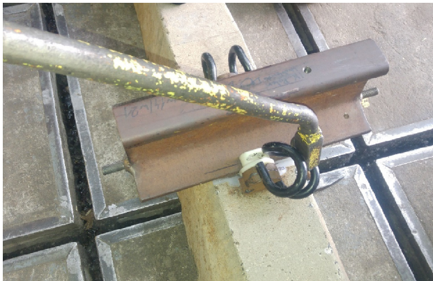
Fig. 2. SB4-type spring clip assembly strength testing station [authors' own work]
