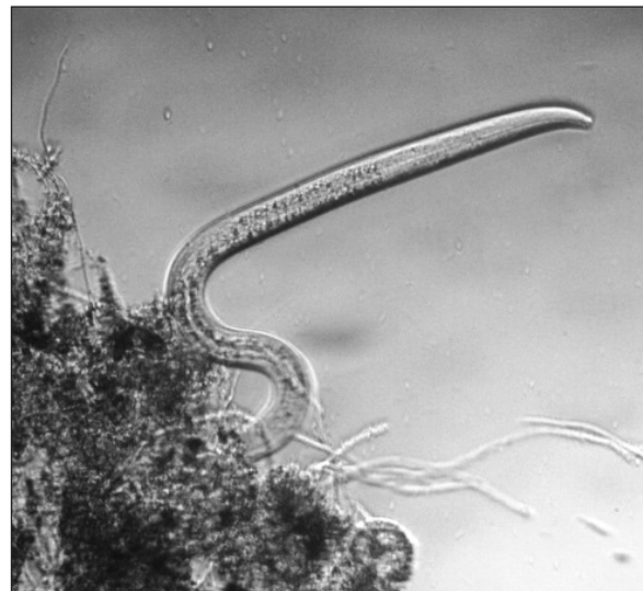
Figure 2. Nematode attached to the floc of activated sludge
