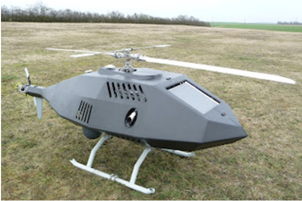
Fig. 1. The image of the remote-controlled Tanan 300 helicopter. The lightweight Diesel engine is applied to drive the machine [the advertisement of the Cassidian company at www.miltechmag.com/2012/08/cassidians-tanan-300-vtol-uas.html ]
