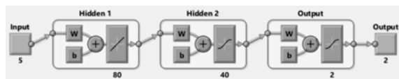
Fig. 15. Architecture of unidirectional three-layer network (neuron activation functions in successive layers: linear, sigmoid bipolar, sigmoid bipolar).
