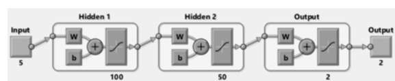
Fig. 14. Architecture of unidirectional three-layer network (all neuron activation functions are sigmoid bipolar). Where: 5 – number of network inputs, 100 – number of neurons in hidden layer 1, 50 – number of neurons in hidden layer 2, 2 – number of output neurons (network outputs), w – weights vector, b – biases vector
