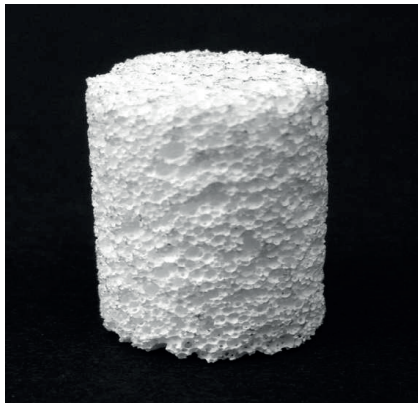
Fig. 1. Cylindrical sample of alumina 90 % porosity foam produced by the chemical method of gelcasting; the diameter amounts 8.0 mm and the height 17.0 mm
