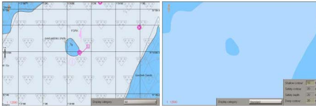
Fig. 3. Extract from ECDIS 3000-i showing alternative display settings for ENC charts for area in question: a) wreck visible; b) wreck not visible [own study]
