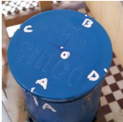
Fig. 5. Designation of a lid whose center point coincides with the center of the guide pipe.
