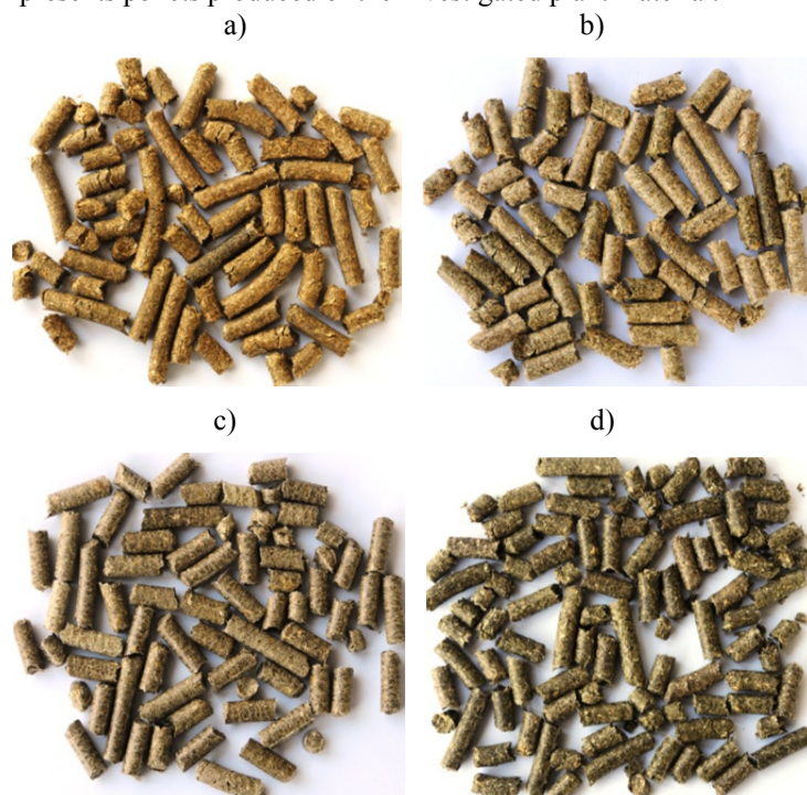
Figure 2. Pellets produced of the investigated plant raw material: a) wheat straw, b) rye straw, c) rape straw, d) meadow hay
