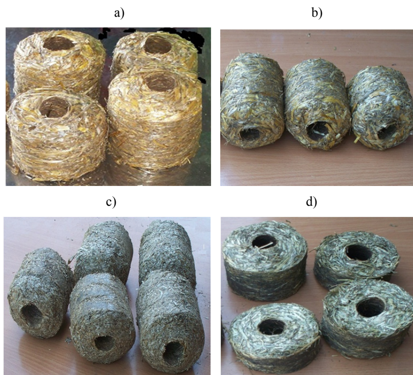
Figure 3. Briquettes produced of the investigated raw materials: a) wheat straw, b) rye straw, c) rape straw, d) meadow hay
