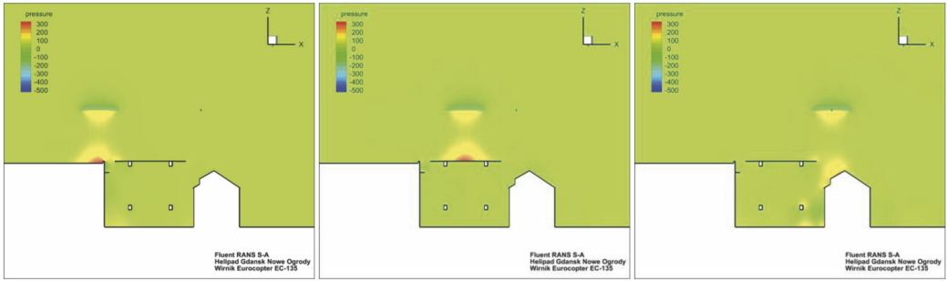
Fig. 11. Static pressure distribution on the W-E cut plane, for cases FAN_W, FAN_C and FAN_E respectively (Dziubiński, 2015)
