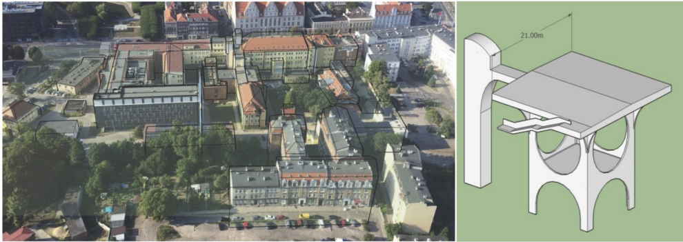
Fig. 1. Comparison of 3d geometry and aerial photography (left) and geometry of planned helipad tower (right) [5]
