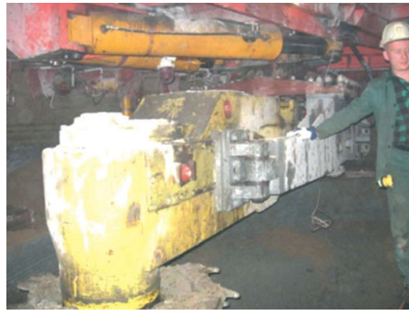
Fig. 16. View of suspension boom of mining head drive system together with head and mining cutter in KDS-2 shaft shearer [9]
