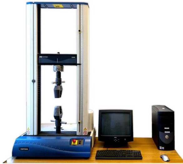
Fig. 10. The test stand for the quasi-static tensile experiments [13]
