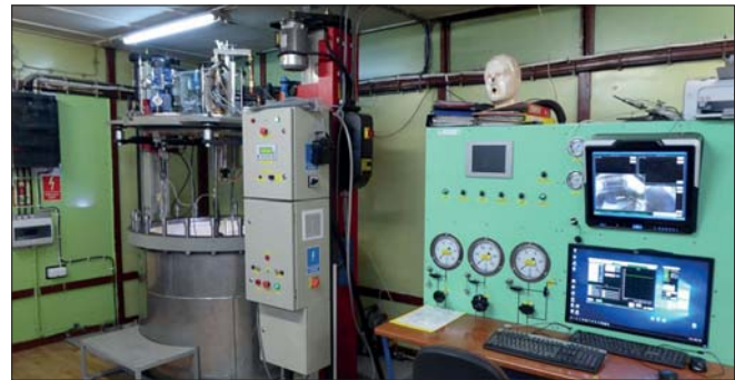
Fig. 5. The set-up of combined simulators: respiratory, metabolic and hyperbaric
