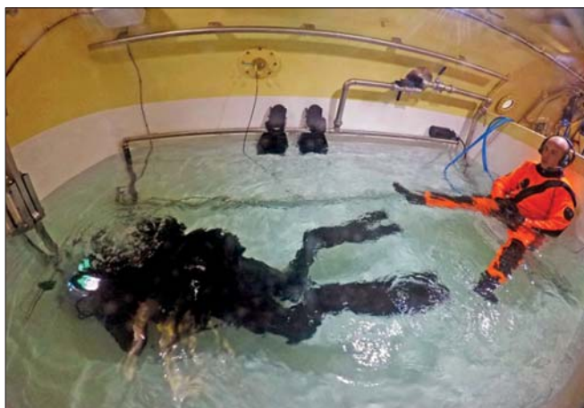
Fig. 7. The hyperbaric swimming simulator
